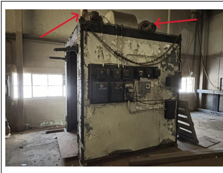
5. "Oven" fixture in center bay of Building 1 with ACM HG12 breaching fittings located on top
