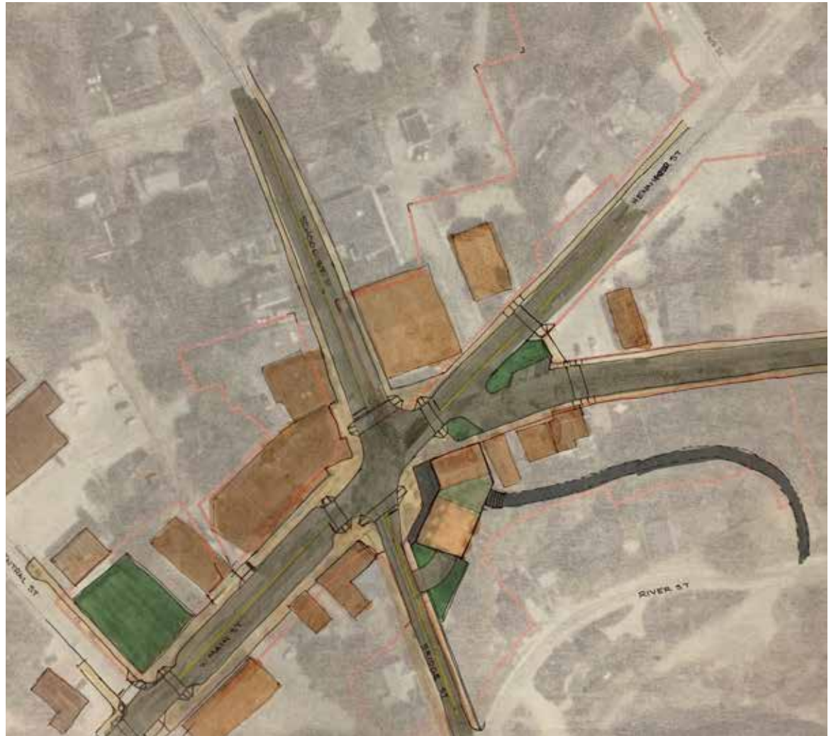
Sketch of potential changes to the flow of traffic, including removing the left turn lanes in order to widen the sidewalks and shorten crossings.
